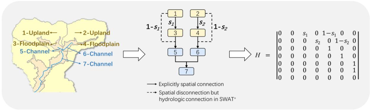
**Fig. 3. Construction of flow distribution matrix  $H$  based on upstream-downstream relationships among landscape position units (LSUs) and channels and flow distribution ratios ( $s_1$  and  $s_2$ ) from upland to floodplain.**
