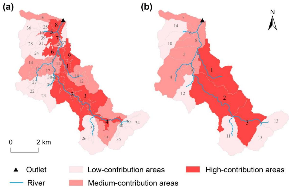
**Fig. 8. Ranking and classification of total nitrogen load contribution at (a) LSU (landscape position unit) level and (b) subbasin level. The labelled number is the ranked sequence of load contribution in descending order. High-contribution areas are identified as PMAs.**
