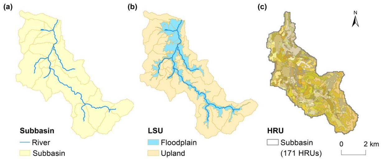
**Fig. 5. Delineation of three types of spatial units in the SWAT<sup>+</sup> model of Zhongtianshe: (a) subbasin, (b) LSU, (c) HRU (take one subbasin as an example). Each color within the same subbasin in the map of HRU represents one unit, i.e., a particular combination of land use, soil type, and slope classification.**
