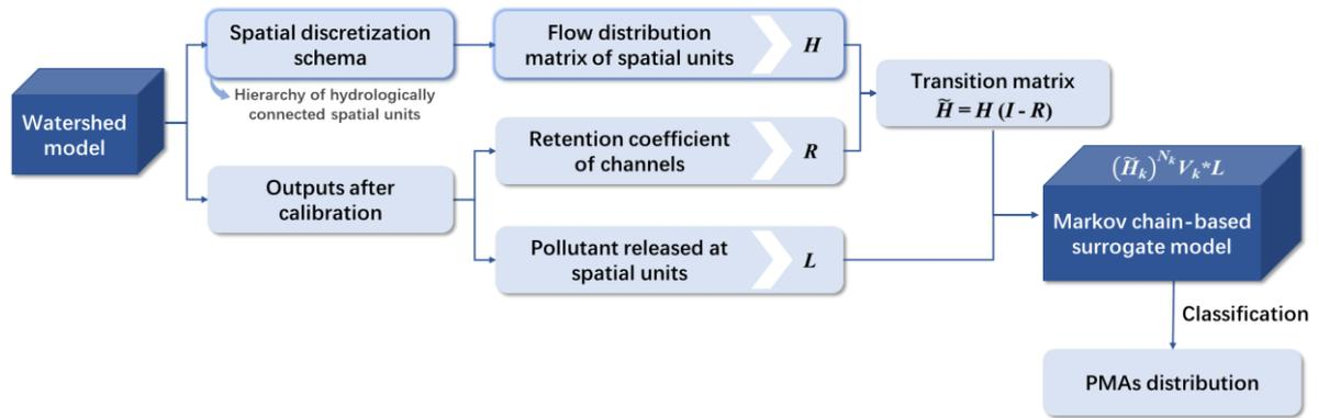
**Fig. 1. Framework of the Markov chain-based PMA identification method using a hierarchy of hydrologically connected spatial units.**
