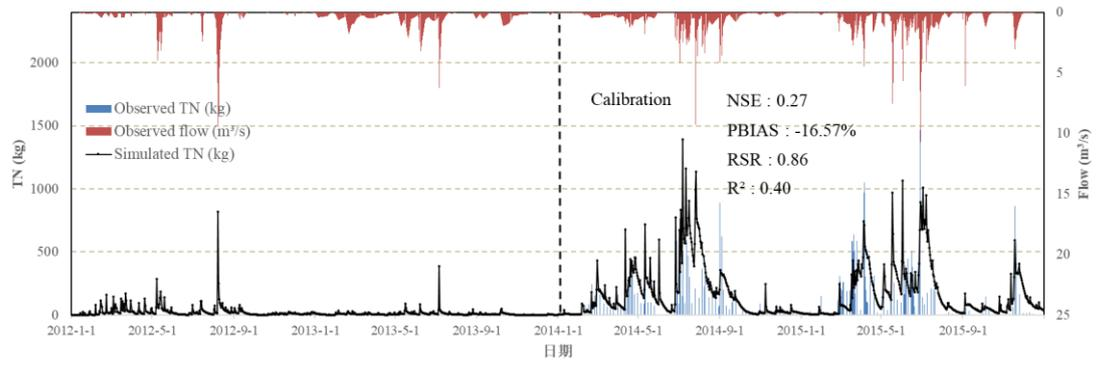
**Fig. 7. Simulated and observed total nitrogen (TN) at the calibration period.**
