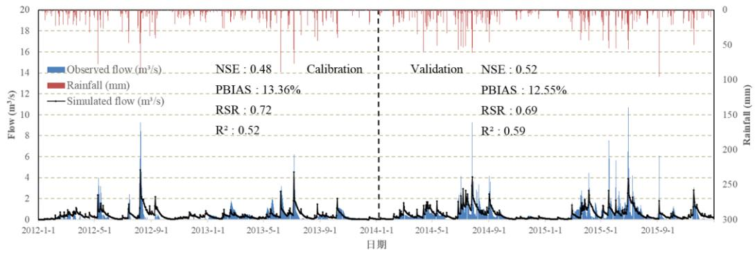
**Fig. 6. Simulated and observed stream flow during calibration and validation periods.**
